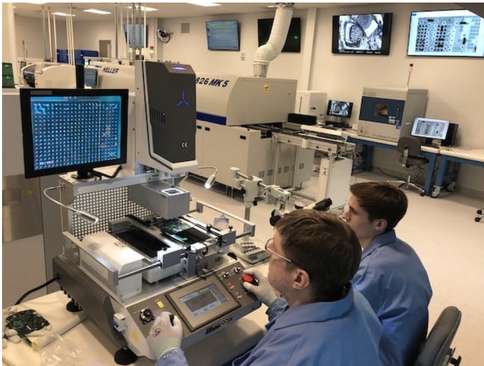
Trainees use X-ray microscopes and an SEM to determine defects in a BGA placement before using the BGA rework equipment to repair the PCB
