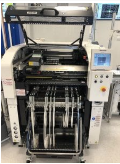
The Panasonic NPM-W2 high-volume SMT pick & place unit can hold up to 60 feeders in the front and 20 feeders in the back with 24 JEDEC trays
