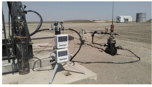
The **Sure Shot Continuous Fluid Level Surveillance System**, provides a cost effective, simple and robust method to measure and tend annular fluid level data for well production maximization, while simultaneously assuring downhole over-pumping risks are controlled.
