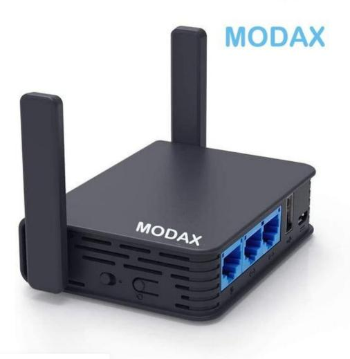
[MODAX] Gigabit Travel AC VPN Router, 300Mbps(2.4G)+433Mbps(5G) Wi-Fi, 128MB RAM, MicroSD Support, Repeater Bridge, OpenWrt/LEDE pre-Installed, Cloudflare DNS
