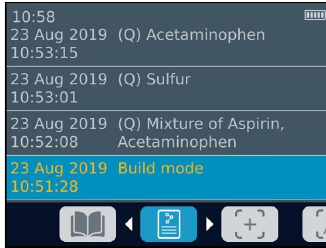
Figure 14. The Review screen shows all measurements taken since the most recent power-on.
