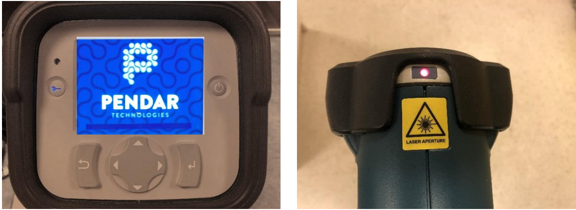
Figure 3- The ARM key (left) and laser emission indicator are illuminated when the system is in READY state.
