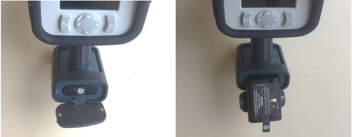
Figure 2. (left) Pull gently on the tab to remove the battery. (right) Slide the new battery into the compartment with terminals facing up.
