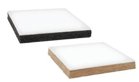
ALP X-Slide<sup>™</sup> and Iso-Slide<sup>™</sup> bearing pads are manufactured with a Polytetrafluoroethylene (PTFE) sheet permanenently bonded to either an Isoflex<sup>™</sup> or X-CORD<sup>™</sup> bearing pad to create a bearing point with a low coefficient of friction, but high bearing capacity. A polished stainless steel plate is attached to the bottom of an upper bearing element to maintain the low coefficient of friction with this system.
