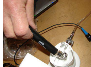
Install the Sensor to Flow Cell
