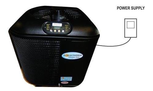
• Determine sealtight length and slip plastic adaptor over conduit. Run conduit and proper size wire from power supply to the unit's main contactor located on the right side of high voltage compartment. The ground wire connection is located on the base of the box to the left of the contactor. A knock out is located on the bottom of the box just below the contactor. A sealtight fitting must be used to attach the conduit to the electric box.
