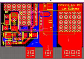
PFC with transition-mode controller L6562A (Top View)
