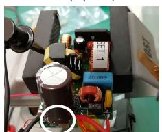
PFC with transition-mode controller L6562A (Side View)
