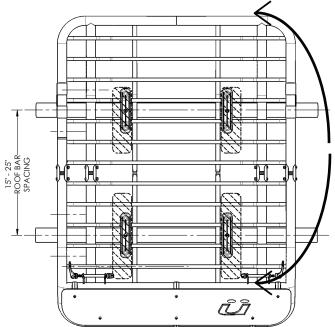
Visor will need to be pivoted down to mount to front bar. Remove top 3 visor clamps to pivot. Visor will stay attached to basket.
