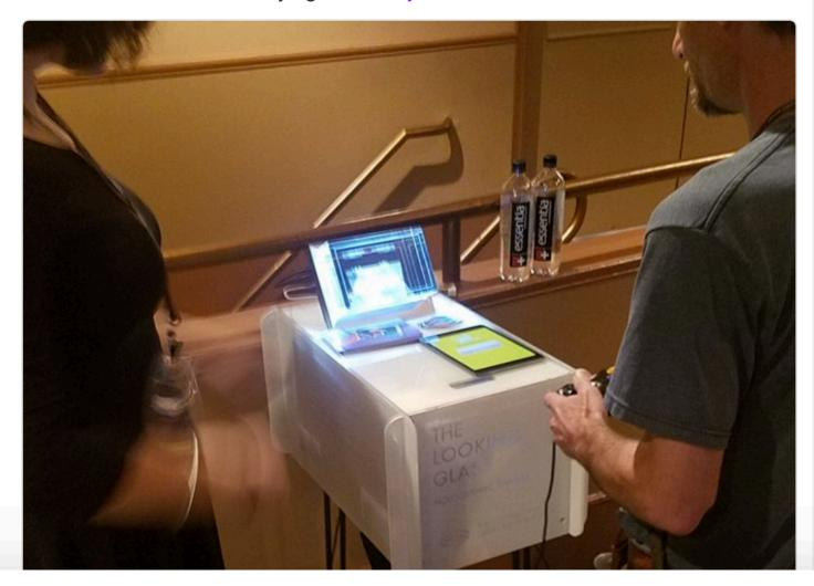
foil and an arduino to sense hand position in 3D space. Now controlling a little spaceship in One of the most mind-blowingly cool 3D controllers we've ever seen, using a few pieces of a L3D Cube at the Taipei Hackerspace!
