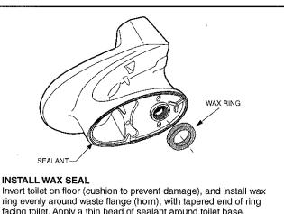
Invert toilet on floor (cushion to prevent damage), and install wax ring evenly around waste flange (horn), with tapered end of ring facing toilet. Apply a thin bead of sealant around toilet base.
