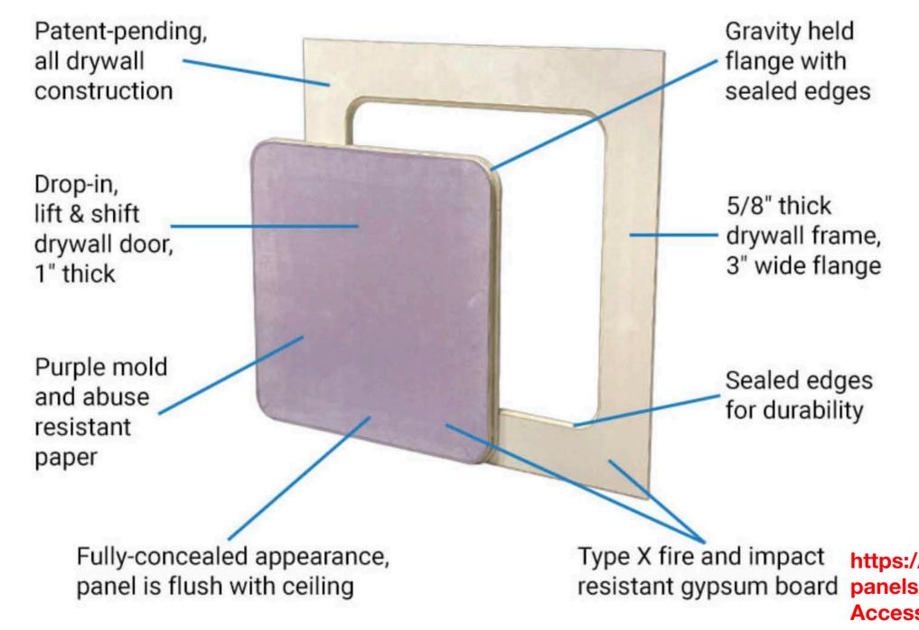
Type X fire and impact https://www.wbdoors.com/product-category/access-doorsresistant gypsum board panels/drywall/wb-dw-405-phantom-series/ Accessed 12/19/2022
