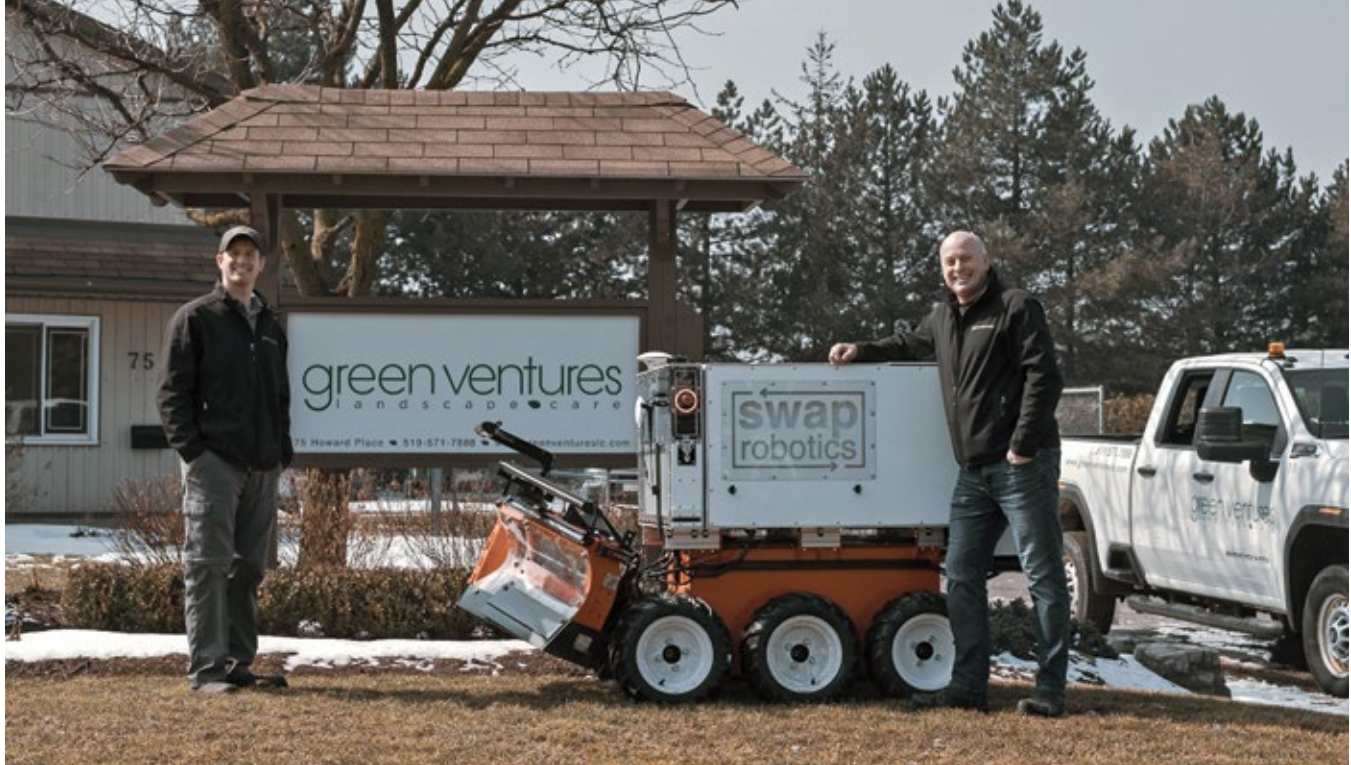
Ryan and Sean Hebel stand next to a battery-powered, semi-autonomous tractor. The machine is used for cleaning sidewalks in the winter. In the summer, switching out the blades for a mower deck spares staff from the hot work of cutting grass in parks.
