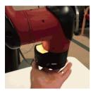
An impedance control example with low stiffness along vertical direction.
