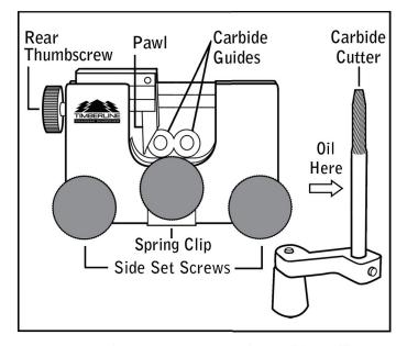
For smooth operation use a drop of bar oil on carbide cutter shaft.
