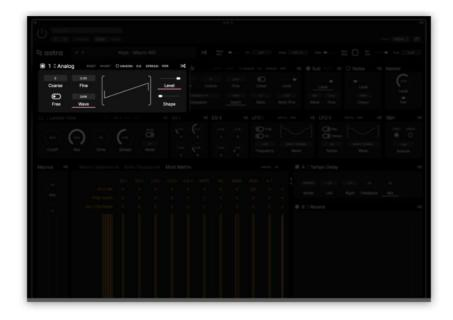
**FM:** The FM oscillator has four carrier waveforms, with a user-loadable main modulator waveform and switchable linear / exponential FM for a wide scope of sound design.
