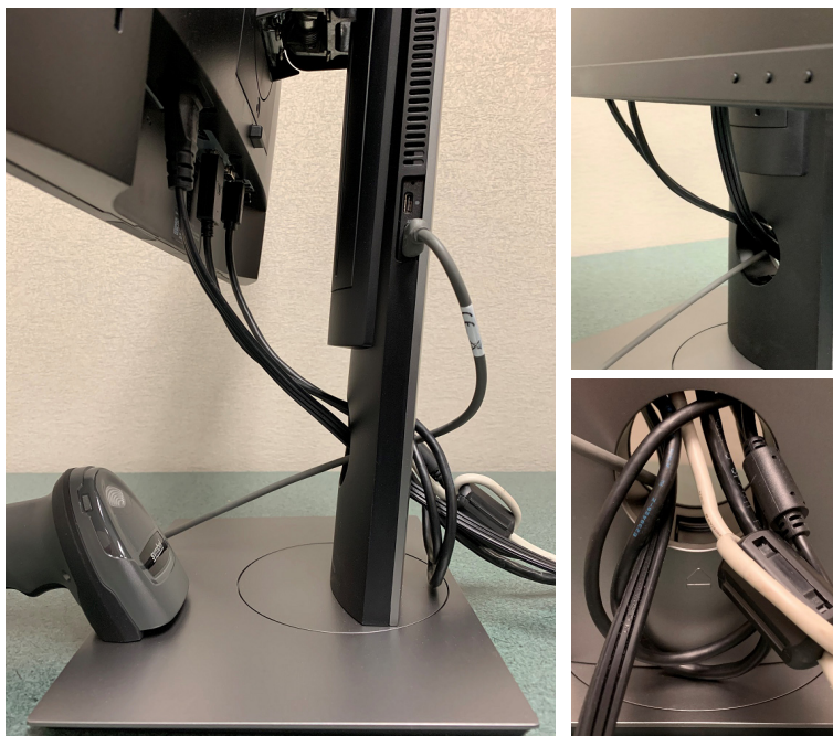
Figure 1-7: Clockwise: Side, lower front, lower rear (showing both monitor cables from the PC coming out the back looped once around the Ella cables and then out the front to monitor).
