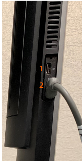
Figure 1-6: Monitor stand side view showing Barcode scanner and optional LAN (adapter not shown) interconnections.
