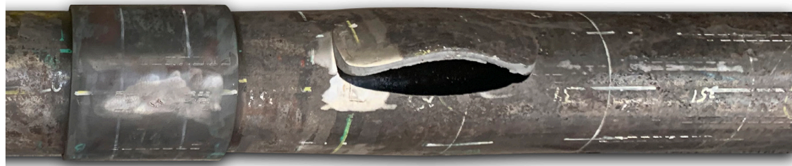
Laboratory test – 5 1/2" 20.00# P110EC Pipe body rupture 19,409 psi, 731 KIPS, no leakage or connection failure at 123% of pipe
