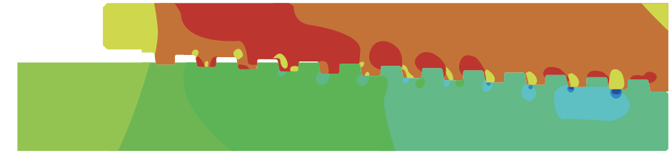
Torque shoulders and thread form optimization provide higher torques and reduced hoop stresses in made-up connections.
