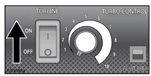
**NOTE:** ProContractor and ProComp models in SmartStart setting will automatically turn off when not actively spraying. Sprayer will start upon re-triggering of HVLP Edge II Plus gun. Turn switch to ON position if SmartStart is not desired. In ON mode, unit will still shutdown after 3 minutes of non-use. Sprayer will start upon re-triggering of gun.
