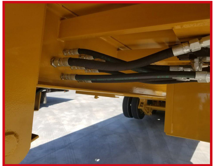
HYDRAULIC HOSES CAREFULLY THREADED THROUGH MAIN BEAM TO PREVENT CHAFFING
