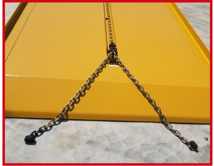
CORNER CASTING CHAIN TO PULL CONTAINERS ONTO THE STEEL DECK
