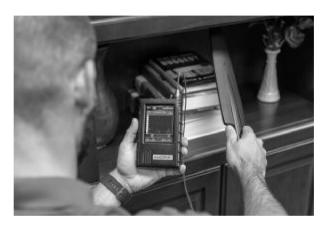
Here the ANDRE Whip/Dipole antenna probe is used to sweep a bookcase in search of hidden transmitters.
