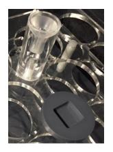
Place empty sample racks in each of the three sample rack positions. There should be NO sample tubes in the sample racks.
