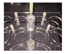
After the aligning the wash cup and clicking/tapping Next Step, the instrument will automatically calibrate the Z-axis position of the probe to the bottom of the wash cup. (the spindle will move up and down and the red light will turn on and off). **MTP well alignment:** Align the center of the probe needles to the center of each indicated reaction plate or predilution plate well:
