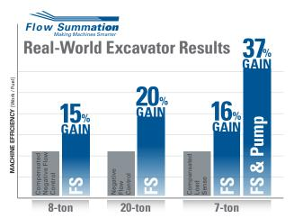
The graph above represents actual machine improvements by upgrading from competing systems to Flow Summation valve technology and the respective gains in efficiency these improvements have created.
