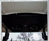
The Plug & Play Overhead Audio Console for Drive2 arrives ready to install and includes a Bluetooth amplifier and speakers housed in a powder coat painted, form fitting aluminum console. See page 209 for details.
