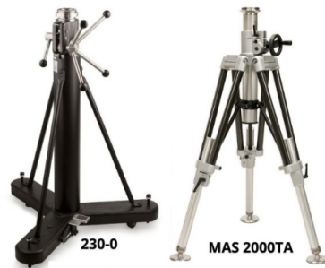
Metrology stands for KinAiry laser tracker field test
