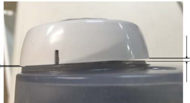
Uneven spacing around the perimeter
