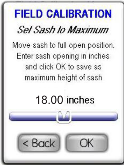
Fig 7. Set sash to maximum position and enter the height to complete the calibration procedure.
