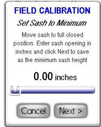
Fig 6. If sash position sensor is connected, it must be recalibrated following installation.
