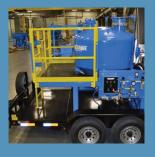
The **SandAlong** is a durable, trailer-mounted unit with the ability to get your sand to a remote locomotive.
