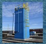
The **SandMaster**™ is a self-contained, single- or dual-position sanding station that delivers traction sand directly to a locomotive sandbox.
