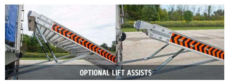
Only Randall Access's Lift Assist combines dual gas shocks and compression springs that ease the ramp up and down. And, only Randall Access carries two Lift Assist options – short and long – to accommodate variances between the enclosure box and trailer floor that are less or greater than 11".
