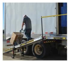
With a 2,000 lbs. capacity drivers can attach a ramp to the platform or use the portable ladder to access the trailer.
