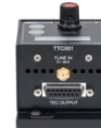
Click to Enlarge Back View of the TTC001 T-Cube (See the Pin Diagrams Tab for More Information)
