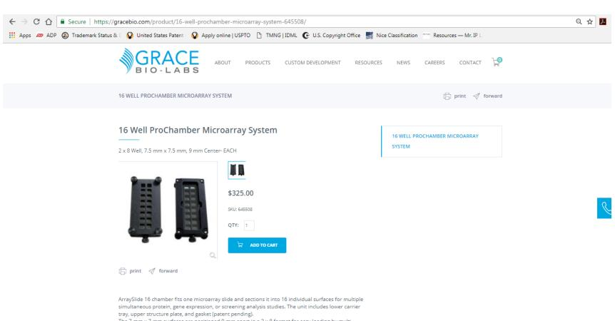
The 7 mm x 7 mm surfaces are positioned 9 mm apart in a 2 x 8 format for easy loading by multichannel pipettes or automated robots. The chamber itself is made from a durable, flat, precision machined aluminum to ensure proper slide alignment and leak-free arrays.
