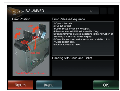
Maintenance guidance screen
