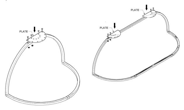
**Step 5:** Attach R2, R3, R4, R5, R6,R7 to top plate. Use self tapping screws to secure the ribs to LPR and RPR. Note: For Larger Awning, connect center rib to TB and FB. You will also need to attach wall supports (WS) to the center of the FB (not shown)
