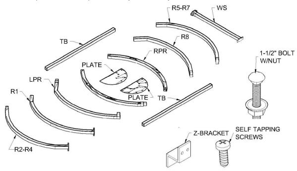
**Step 2:** Connect R1 And R07/R8, and Connect LPR and RPR. You may need a rubber mallet to set the tubing into the fittings. Secure with Self tapping screws.
