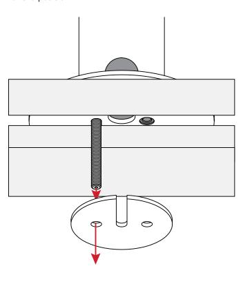
Insert the wing screw into the empty hole on the underside of the riser via the hole in the circular mounting plate. Tighten the wingnuts onto the posts.
