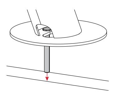
2 From the underside, slide the circular mounting plate all the way over the post with the gap facing the front of the position.
