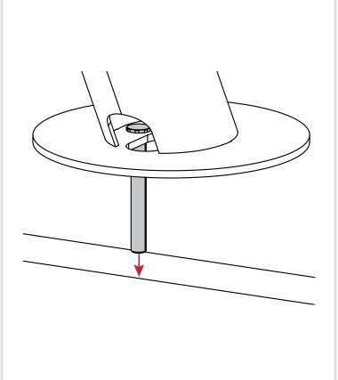
From the underside, slide the circular mounting plate all the way over the post with the gap facing the front of the position. Tighten the wingnuts onto the post.
