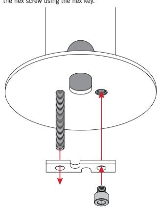
2 Place in the slot on the fixture.
