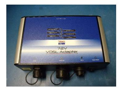
When the unit is first powered on, the Power LED will illuminate.
