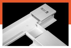
Most runs will go in one direction. But when you need to change direction, EcoTray™ can accommodate. EcoTray™ is cut easily with a hacksaw or a reciprocating saw. Make some simple cuts, insert a plastic rivet, and you will have a secure and stable T-fitting or elbow. A file or deburring tool quickly gets rid of sharp edges.
